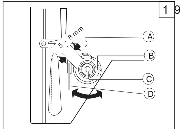
20 . Adjusting the tension of needle thread &
