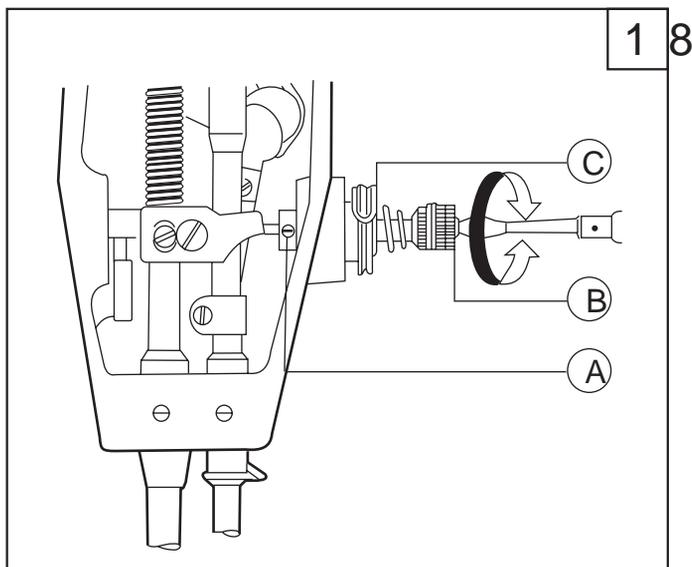
thread take-up spring(C) to zero, and to turn tension stud (B) clockwise until spring (C) just comes into contact with the stop slot on the thread take-up spring regulator, then to further turn tension stud (B) counter-clockwise by 1/2 turn After adjustment, tighten tension stud set screw (A).
