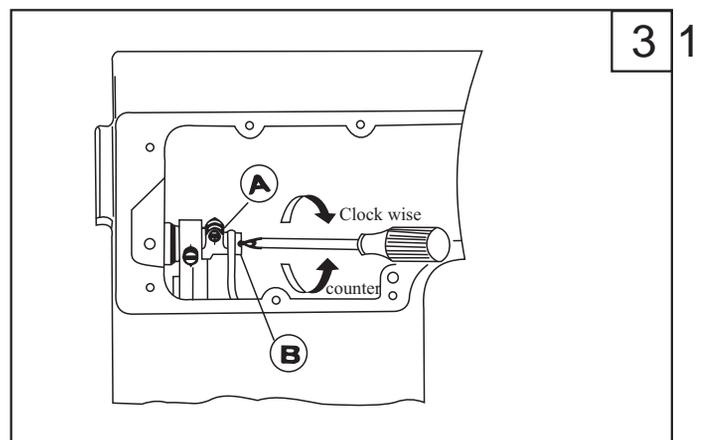
26. Feed timing and adjusting (Fig 32)
