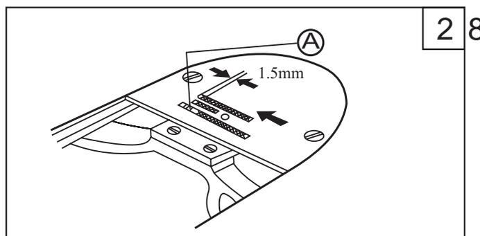
To adjust the position of feed dog, move feed dog to the front end of throat plate, Loosen Screw A (See Fig 29b), move feed dog support B in the direction shown by arrow (Fig.29a) to adjust. After adjustment tighten Screw(A).
